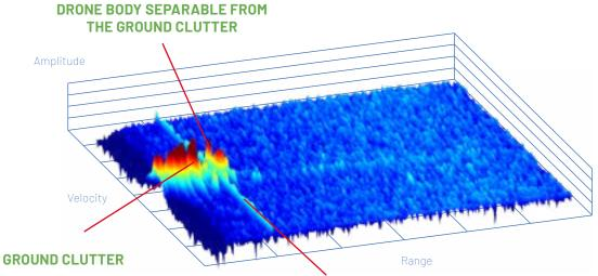
**DRONE PROPELLERS DETECTED**
