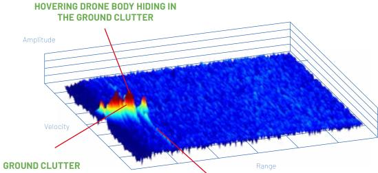
**DRONE PROPELLERS DETECTED**
